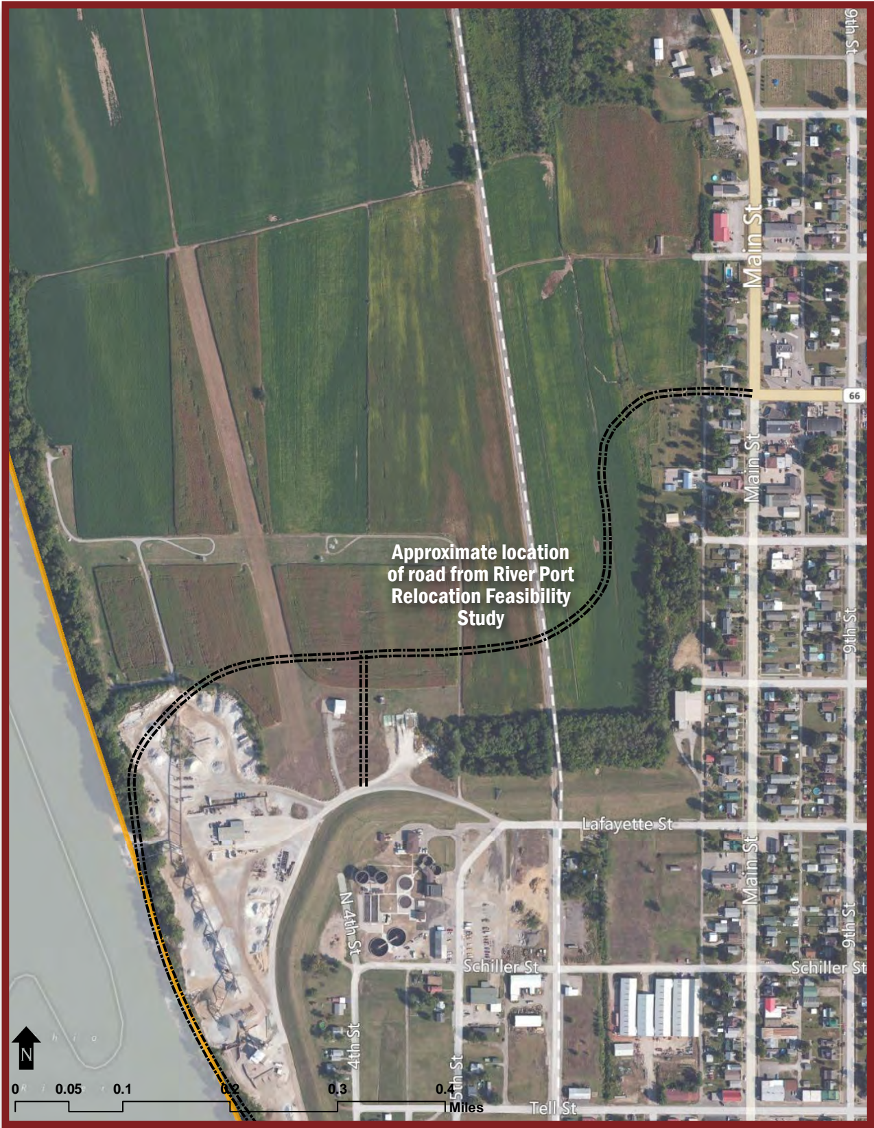
Figure 14: New Road Alignment from River Port Relocation Feasibility Study
